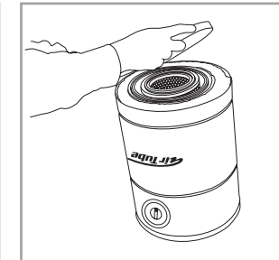
Step 3 Remove lid by pulling slightly on cover.
